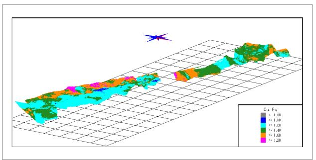
Figure 1-1: Knife Lake Deposit 3D View- Modelled Blocks showing Cu Eqv. Grade – looking Northwest
